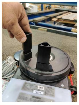
The motor package includes legs, bolts and washers; insert the legs as pictured. Drop in washers and then screw in the bolt until tightened.
