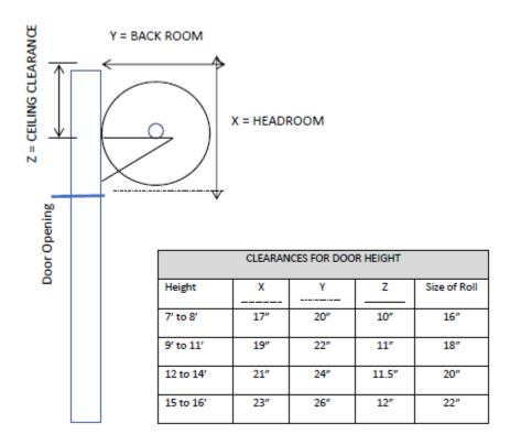
**DOOR SIZE – Width**: The door curtain should be 4 inches wider than the opening. However, a wider than normal door can be fitted by allowing the door to overlap further on each side, providing the additional side room is available.
