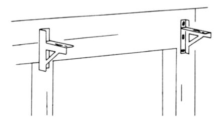
The curtain is made 4 inches wider than the opening – to overlap opening on each side by 2 inches
